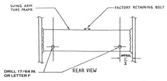
3) 'Skin sharpen' the drill by grinding it flat across the tip, or buy a skin sharpened drill at a tool supply house. Using this drill, bottom out the holes against the spindle. There will still be a small burr at the bottom of each hole, but this is OK.
